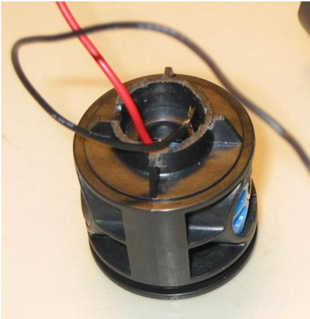
Slot the switch assembly back into the housing and use the allen key to tighten the set screw to 'fix' it back where it should be. Replace the rubber boot.
