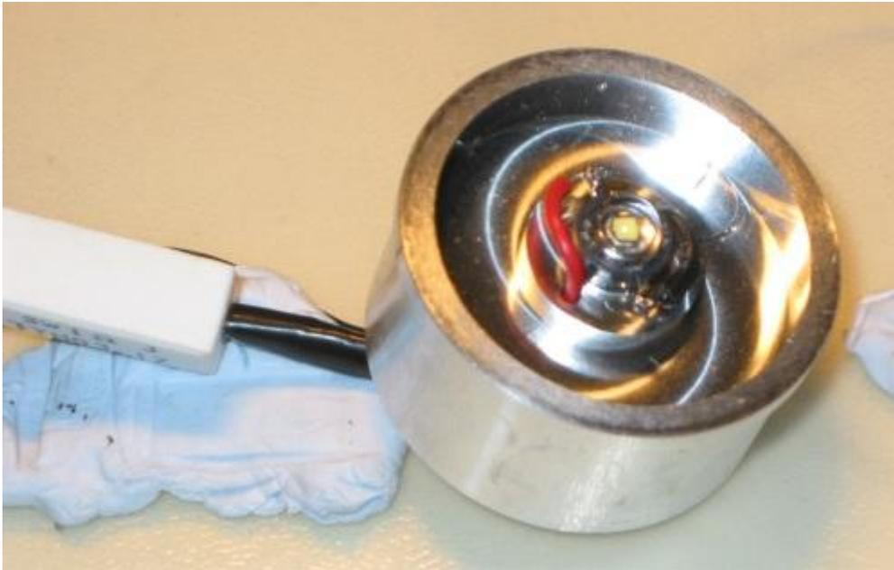
Note that the side with the "O" designates [CHECK AND CONFIRM from datasheets]. Connecting the Lux in reverse will result in nothing lighting up - a diode needs its polarity to be correct. Been there done it on another one of my mods.. sheesh.
