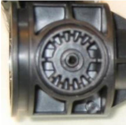
Once the set screw comes loose, the housing should simply drop out of the bottom of the tubular housing. You may need to apply a little bit of pressure on the bulb end to get it to come out.
