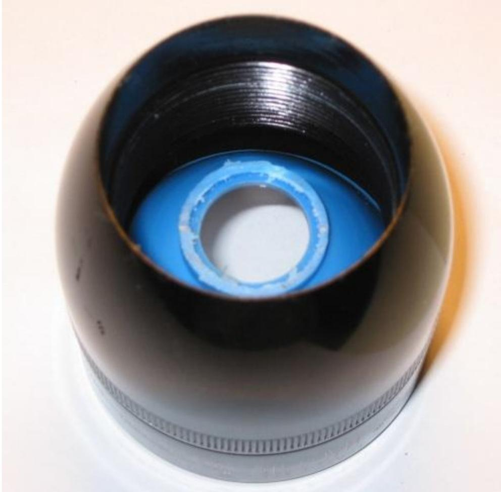
Now, fit the Hotlips into the center of the aluminium housing, pushing the resistor and the wires in. According to Hotbeam you may need to sand the interior of the aluminium housing if the Hotlips does not fit. Mine fits perfectly, provided I align it properly. You must be dead level with the tube, before it slips in with some gentle pressure.
