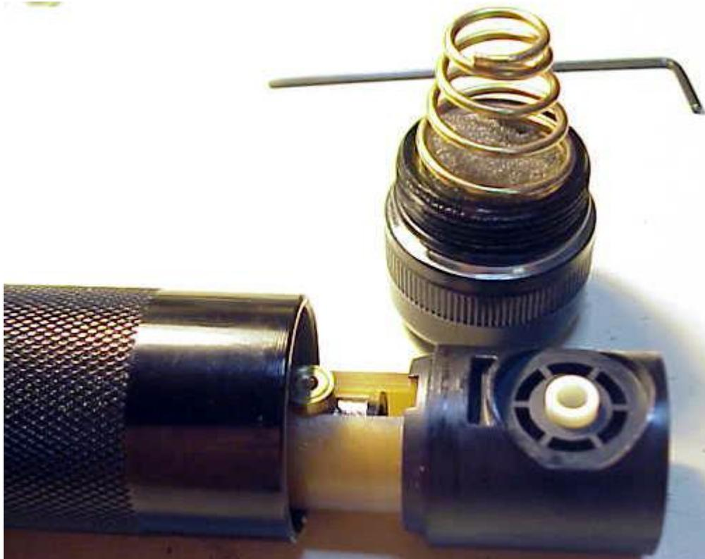
Use the same key to unscrew the focusing wheel and remove all the metal internals and discard (hint - push down slightly on the bulb to relieve pressure on the wheel while unscrewing):
