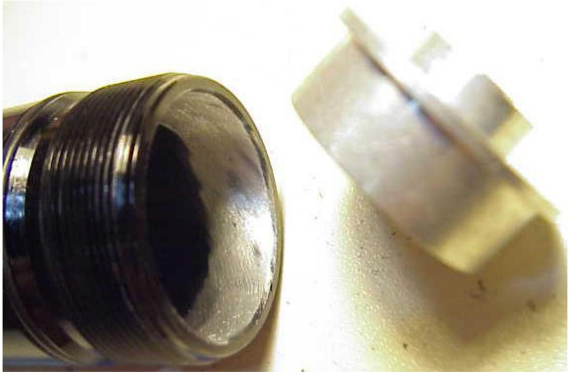
Drop the switch body back down into the tube from the bottom, line up the switch with the hole and tighten firmly:
