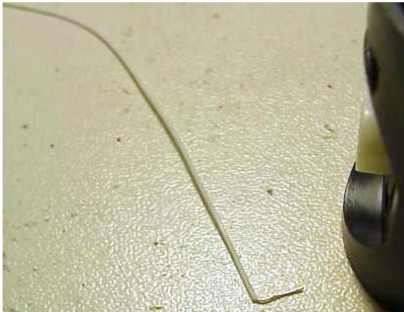
and then stick it down the now-empty tube of the switch body so that the 90 degree stripped end makes flat contact with the metal plate at the bottom. From above, carefully hold the stripped wire tip down against the plate with the flat portion of a chisel-tipped soldering iron and with your other hand, feed some solder line through the side slot onto this joint:
