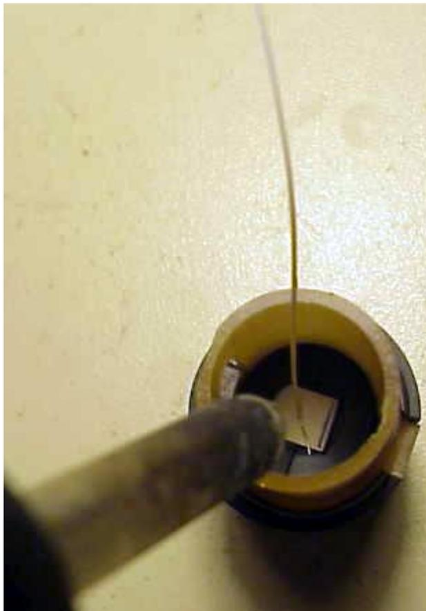
This is the purpose of using teflon jacketed wire; if it contacts the shaft of the soldering iron during this operation the insulation won't melt. As soon as adequate solder flows onto both the plate and wire:
