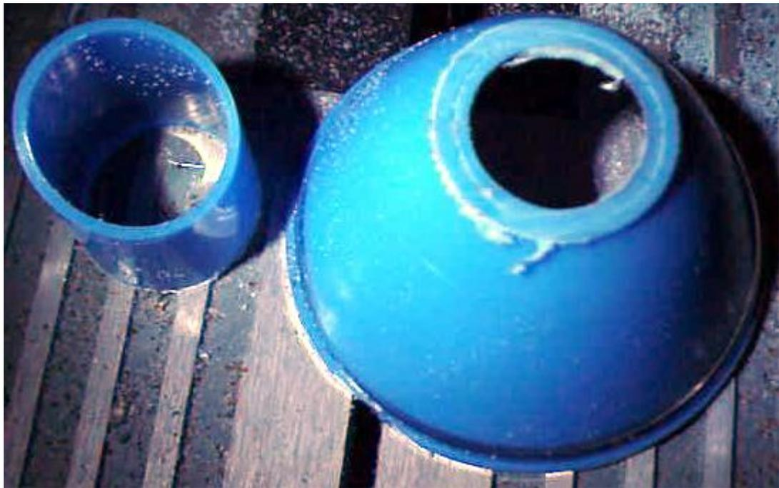
The point here is that the post of the o-ring will fit up into the opening of the reflector anyway so leaving a bit of the "collar" does not hurt. It's not like people (except maybe anally-challenged Flashoholics) are going to look inside there anyhow!
